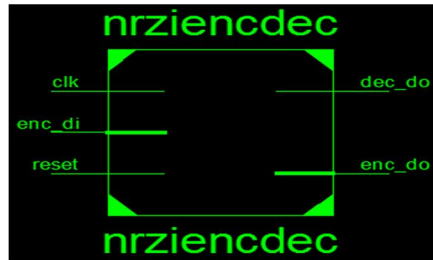
Figure5. RTL schematic symbol of NRZI encode and decode
